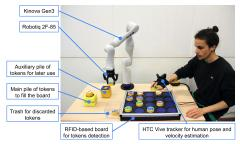
Fig. 4: Setup of filling a tray, the validation task.
